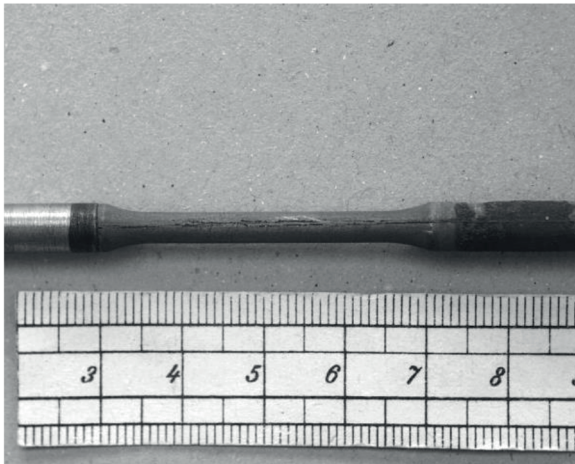
Figure 9 Longitudinal cracks on the X52/AR steel specimen
