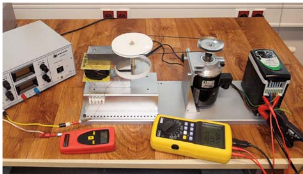
Fig. 7 The setup for measuring the dynamical drag torque of the magnetorheological brake
