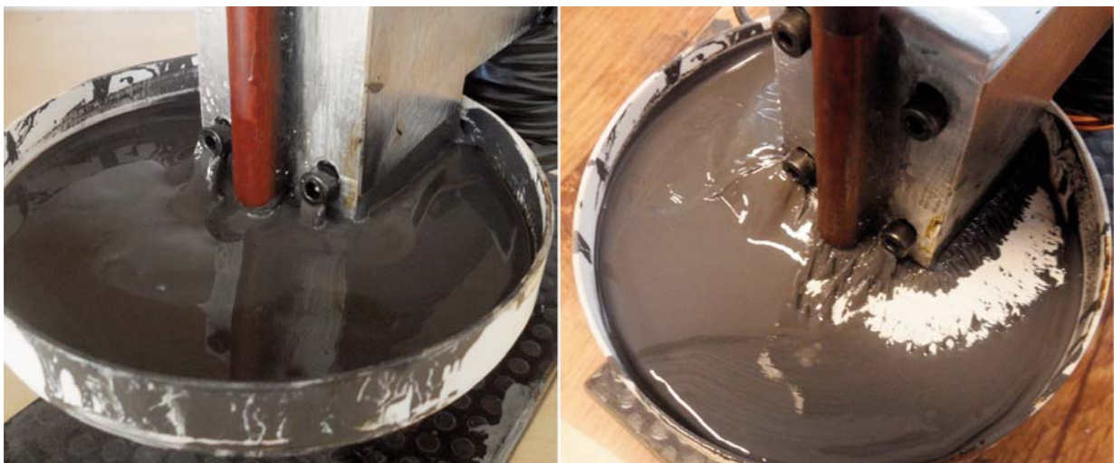
Fig. 6 Magnetorheological brake influences the viscosity of the fluid in the gap: Left - Coils are not powered; Right - Coils are powered with current density of 6 \cdot 10^4 \text{ A/m}^2
