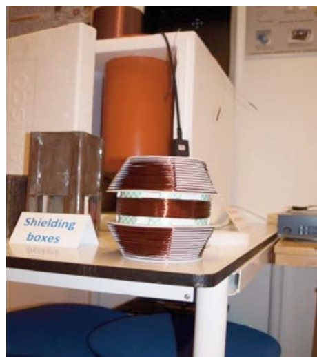
Fig. 5 The finalized exposure coil system in front of the incubator
