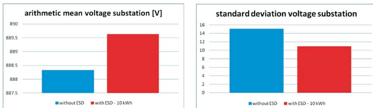
Fig. 12 The average values of voltage at the terminals of the substation and the standard deviation of the voltage without and with ESD ( E = 10 \text{ kWh} ) beyond communication peak driving metro trains
