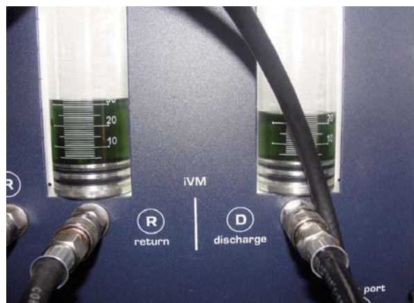
Fig. 1. Examination of the injector with the use of Common Rail injectors diagnostic test stand DS2 by Magneti Marelli
