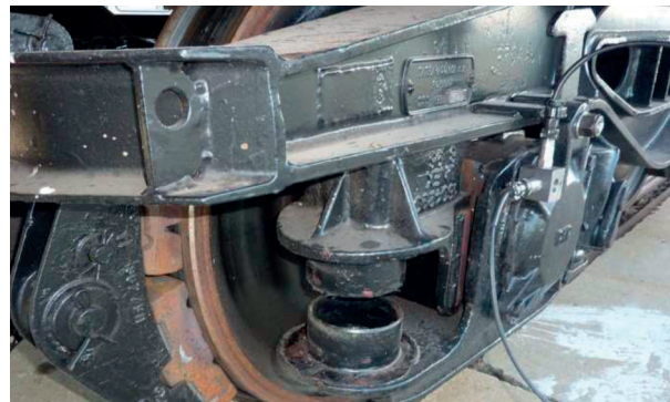
Fig. 4 Freight car bogie with removed springs on one side
