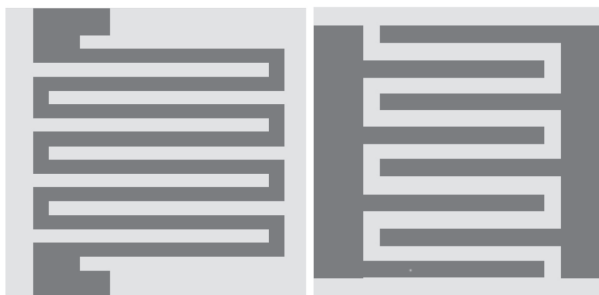
Figure 3 Design of \text{Al}_2\text{O}_3 substrate of the sensor with dimensions 2 \times 2 \text{ mm}^2 equipped with comb electrodes (dark areas, right). Electrodes are composed of 20 nm of Ti (adhesive layer) and 200 nm conducting Pt upper layer. The width of stripes is 50 \mu\text{m} . At the left side, there is a meander for in-situ heating of the sensor. It is patterned on the rear side of the substrate
