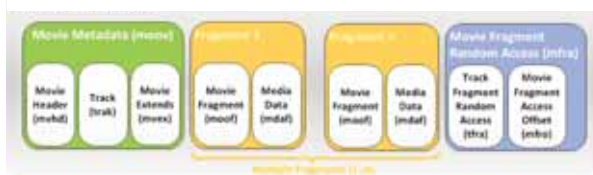
Fig. 9. High level ISO file format structure with multiple fragments used by MS-SSTR [19]
