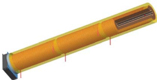
Fig. 8 External and internal structure of borehole simulator
