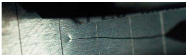
Fig. 9 Plastic zone near crack front during 2.7-times overload, distance between marks being 5 mm
