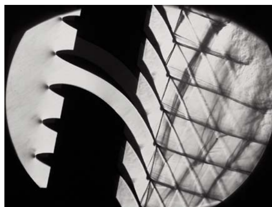
Fig. 3 The schlieren picture of the flow field in a profile cascade, i = 0^\circ , M_{2is} = 1.402 . Additional shock waves appear in the exit flow field which is therefore disturbed and aperiodic
