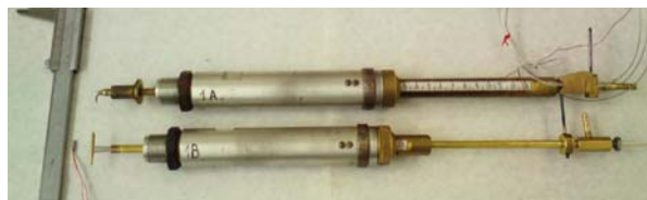
Fig. 5 Original combined probe with thermocouple (top) and new combined probe with bush for platinum thermometer (bottom)
