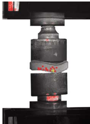
Fig. 3 Tearing of the test specimen
