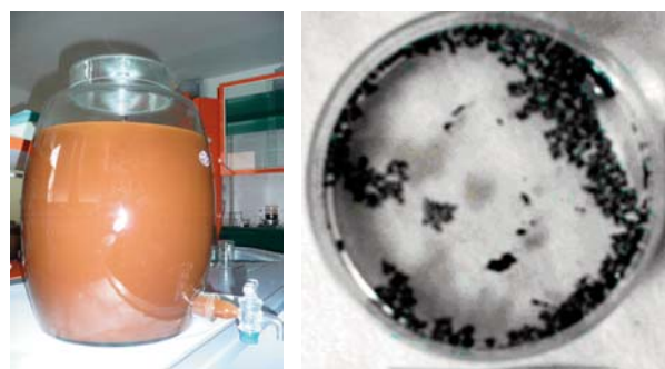
Fig 7 Supply tank with DF water solution in comparison with an insoluble C 60
