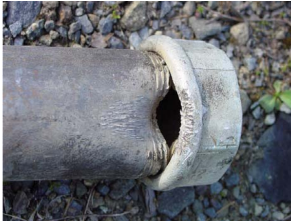
Figs. 13 and 14: Insufficient result of shooting down the end cap
