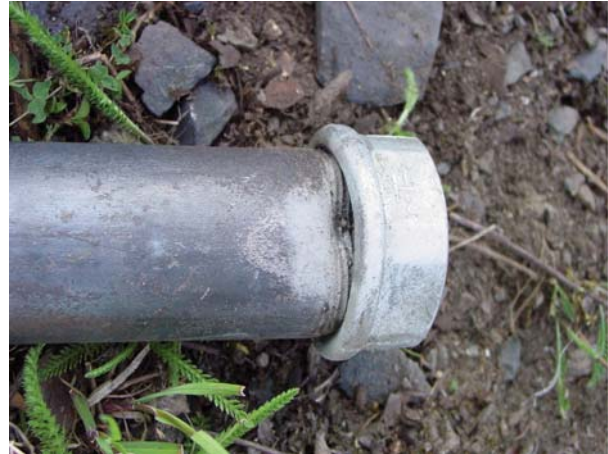
Figs. 13 and 14: Insufficient result of shooting down the end cap
