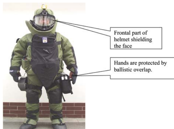
Fig. 1 EOD-8 heavy bomb disposal suit
