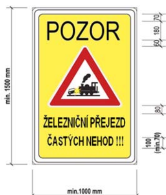
Fig. 2 Design of traffic sign “Caution, frequent accident level crossing”
