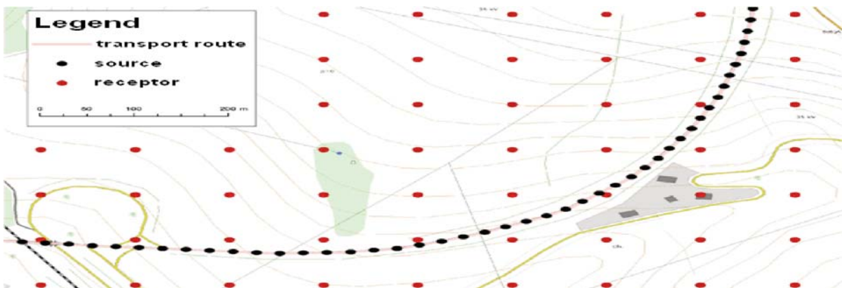
Fig. 4 Schema of segments road distribution and reference point network lay-out.
