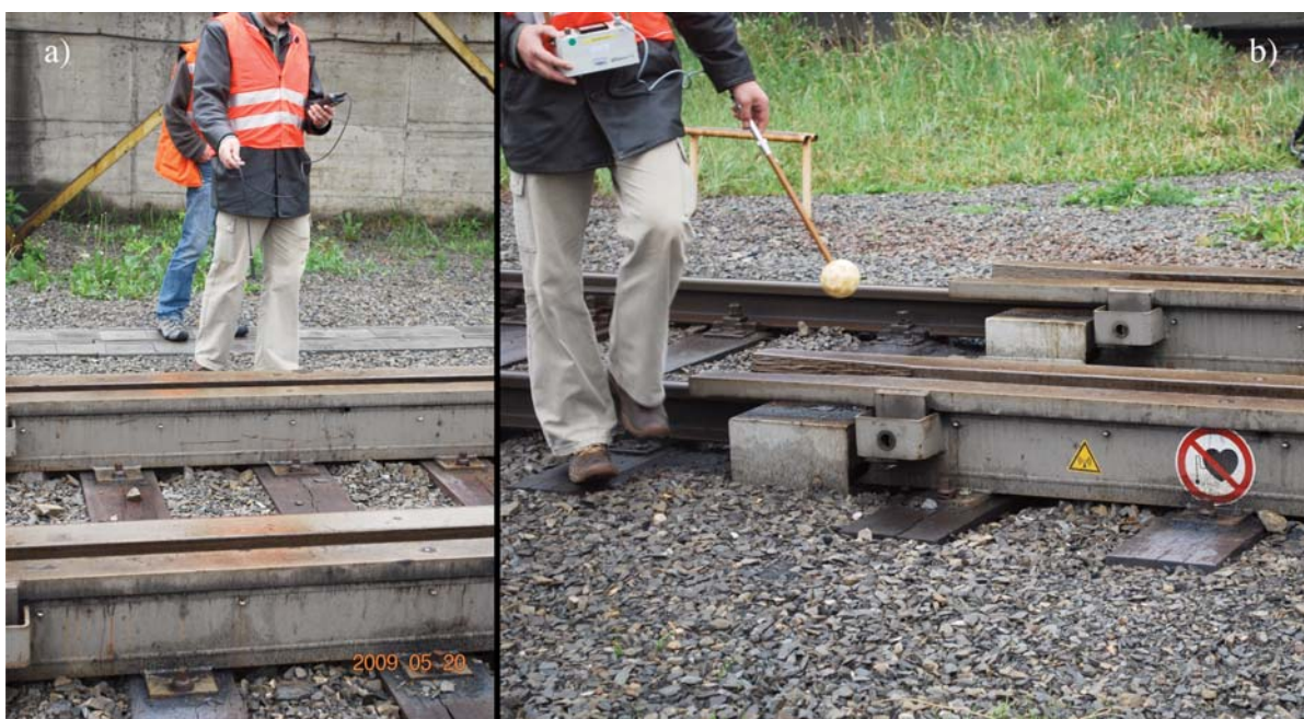
Fig. 7 Measurement of the a) static magnetic field b) rotating magnetic field
