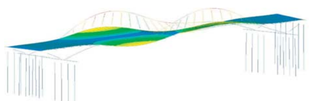
Fig. 2 Frequently occurred natural vibration frequencies f_6 \div f_9 in the tests and their corresponding mode shapes for vibration of the bridge deck.
