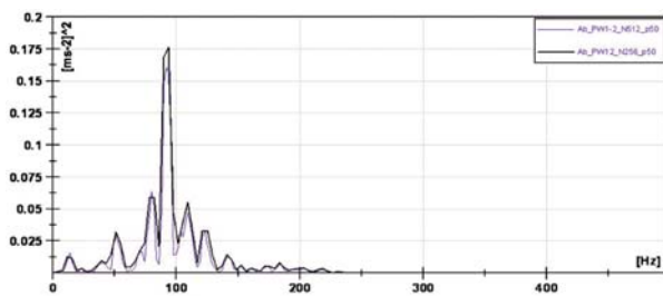
b) LABVIEW Analysis: The PWS of the ballast bed acceleration w''_B(t) /the accelerometer A_B , the passage of coach bogies No.1-2, t = 3.01 - 3.8 = 0.79 s. → the block size N512, overlap 50% - The mean of 2 sp. PWS, → the block size N256, overlap 50% - The mean of 5 sp. PWS. The non-filtering signal for frequencies f = (0 \div 500) Hz.
