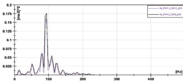
Fig. 10 Analysis of the vertical ballast bed acceleration w''_B(t) /the accelerometer A_B for the passage of coach bogies No. 1-2, t = 3.01 - 3.8 = 0.79 s.
