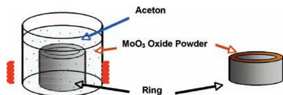
Fig. 3 Sample preparation procedure - coating
