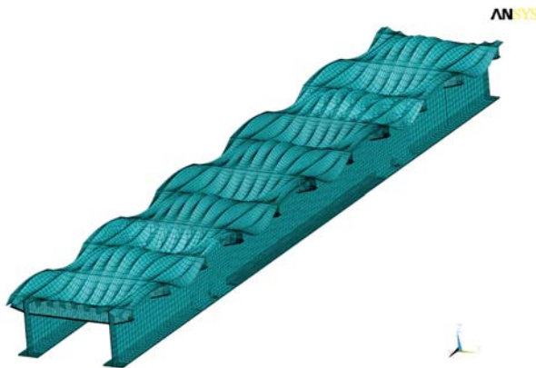
Fig. 1 Deterministic finite element model of orthotropic plate deck - shape of initial deformation (multiplied 100 times) with finite element mesh.
