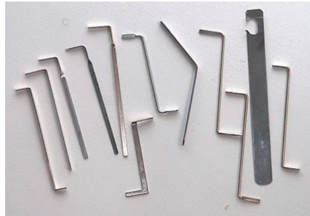
Figure 5 left - Set of various picks and right - tension tools used in lock picking method [8]
