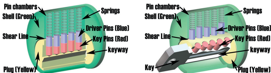
Figure 1 left - Cylinder pin-tumbler lock design and parts, right - rotation of the plug using a key with correct paracentric profile [3]
