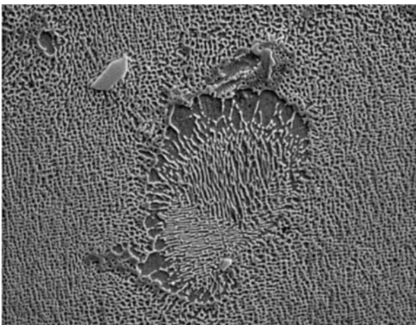
Fig. 11 Precipitation of minority phases after 10000 hours exposition, SEI, magn. 2200x
