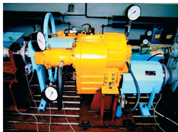
Fig. 2. Gearbox at the test stand
