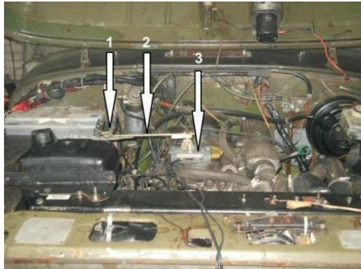
Figure 1 The way of mounting the measurement system in the tested vehicle, 1 - suspension structure of the clamping arm, 2 - potentiometer arm, 3 - linear potentiometer
