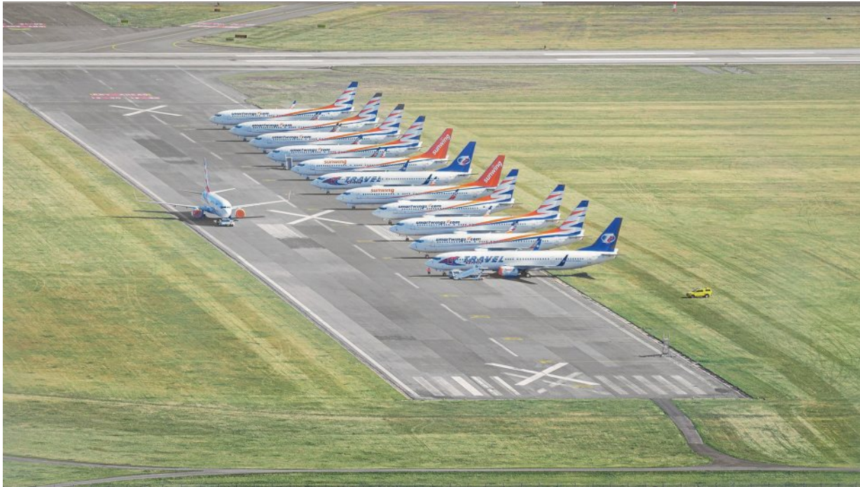
Figure 1 Closed RWY 04/22 at Praha/Ruzyně airport with COVID-19 grounded aircraft parking; marked with 'closed runway marking'; author: Vocelka, T.
