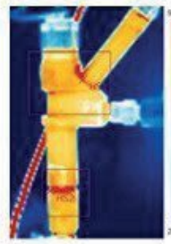
b) thermograms taken from the body of the CR-injector
