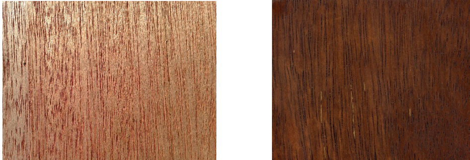
Figure 2 Structure of Meranti (on the left) and Merbau (on the right) [3]
