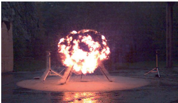
Figure 13 Test of the explosion regularity of Semtex 10-SE, t = 5.236 ms
