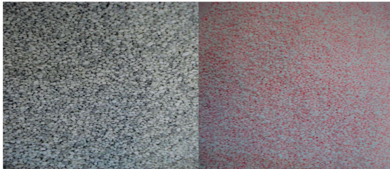
Figure 1 Industrially made explosives DAP - E (left) and DAP - 2 (right) in the prilled form
