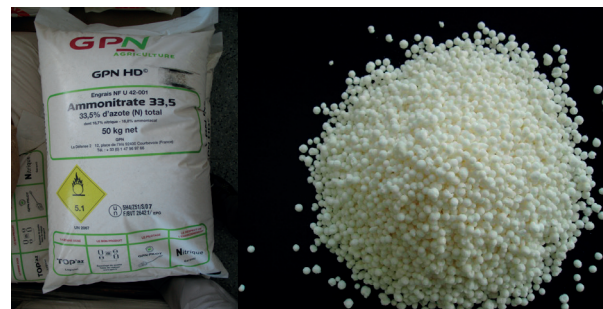
Figure 3 Ammonium nitrate used in the field tests a) sack b) prills
