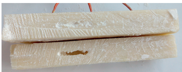
Fig. 9 Shrinkages and cavities in the samples
