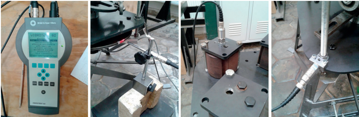
Fig. 8 Measurement device and positioning of RPM and acceleration sensors
