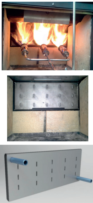
Fig. 7 Evaporator of the loop gravitational heat pipe and its location in the furnace
