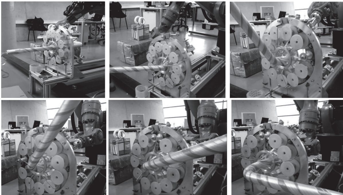
Fig. 8 Time response of real fibre winding process with data from a numerical model
