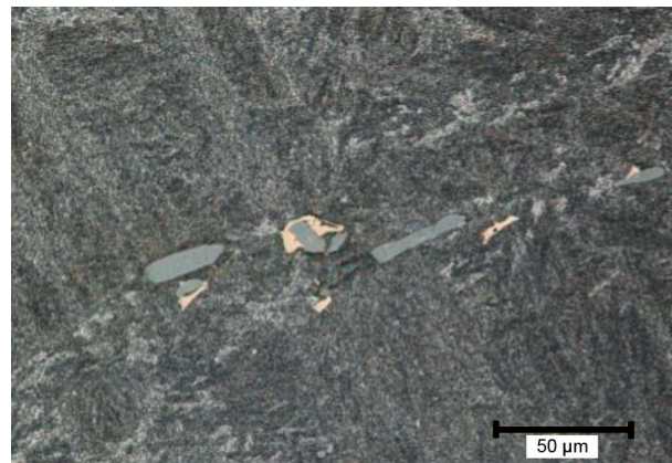
Fig. 6 Microstructure with inclusions
