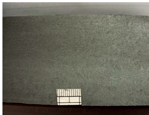
Fig. 2 Macrostructure below the surface
