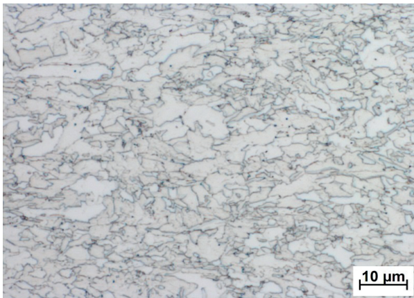
Fig. 1 Microstructure of tested steel STRENX 700MC
