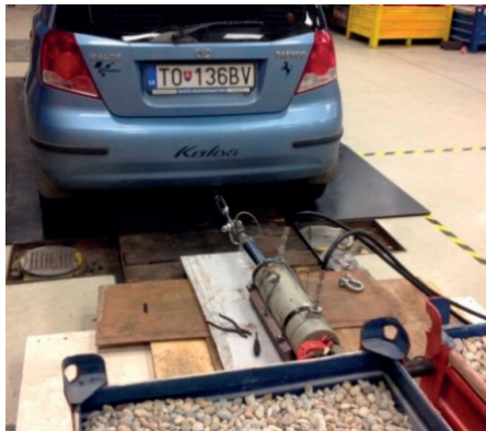
Fig. 3 Connection of the vehicle to the piston by the towing device at the back, Source: Authors
