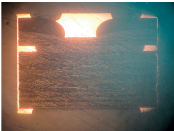
Figure 2 Cross section of four layers PCB made by Iceberg technology with one layer of power line on outer side
