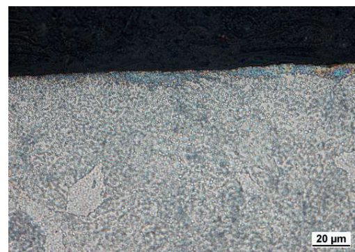
Fig. 4 Microstructure of milled surface, VB = 0.4 mm, HAZ ( 3.6\mu m )
