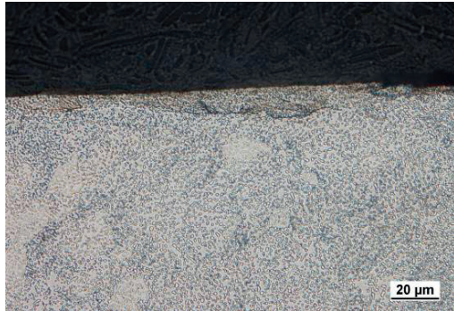
Fig. 5 Microstructure of milled surface, VB = 0.6 mm, HAZ (5 \mu\text{m} )
