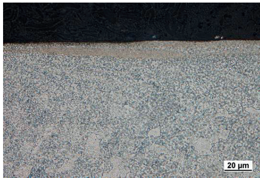
Fig. 6 Microstructure of milled surface, VB = 0.8 mm, HAZ (5.5 \mu\text{m} )
