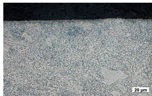
Fig. 3 Microstructure of milled surface, VB = 0.05 mm, HAZ ( 2\mu m )
