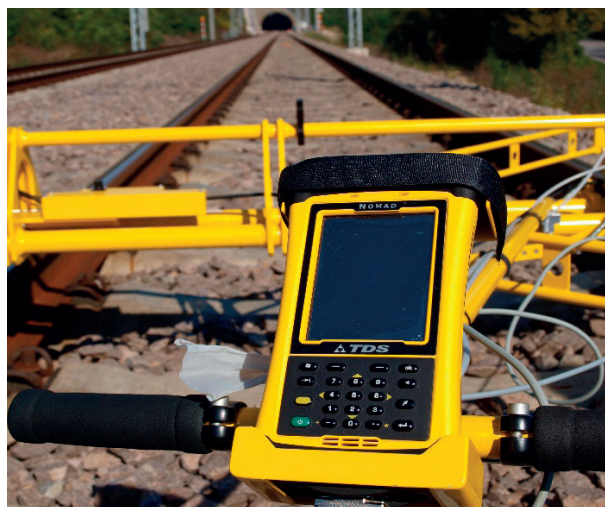
Fig. 2 Continuously measuring trolley KRAB TM -Light (on the up) and computer Nomad (on the down)
