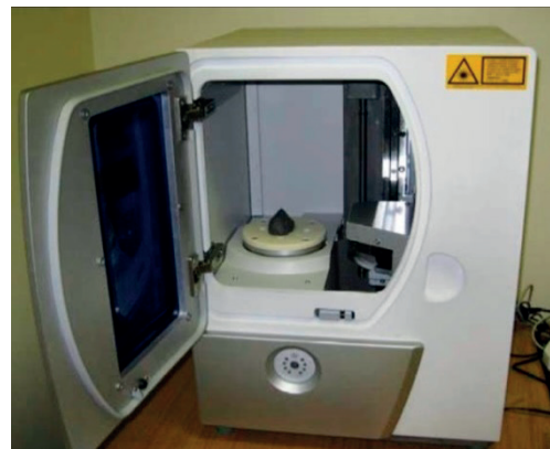
Fig. 4 3D laser scanning device [8]
