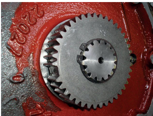
Fig. 6 Sun gear with one missing tooth
