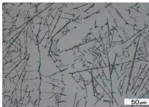
Mag. 200 x and 500x, etching 20 ml H 2 SO 4 + 100 ml H 2 O Fig. 1 Microstructure of alloy with higher amount of iron
