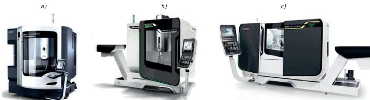
Fig. 1 Analysed machine tools: a) DMU 65 MonoBlock vertical 5-axis machining centre, b) DMC 635 V ECOLINE vertical machining centre, c) CTX 310 ECOLINE numerical control turning centre [26]
