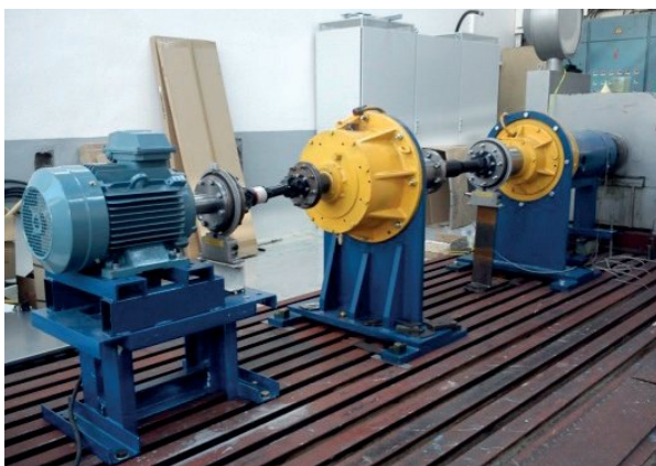
Fig. 1 The testing device used at the Department of Design and Machine Elements for diagnostics of planetary gearboxes' faults (left) and placement of vibration sensors (right)
