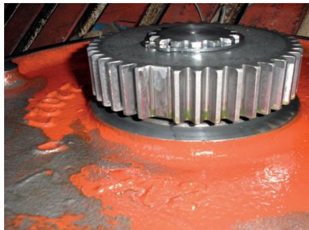
Fig. 6 Sun gear with one missing tooth
