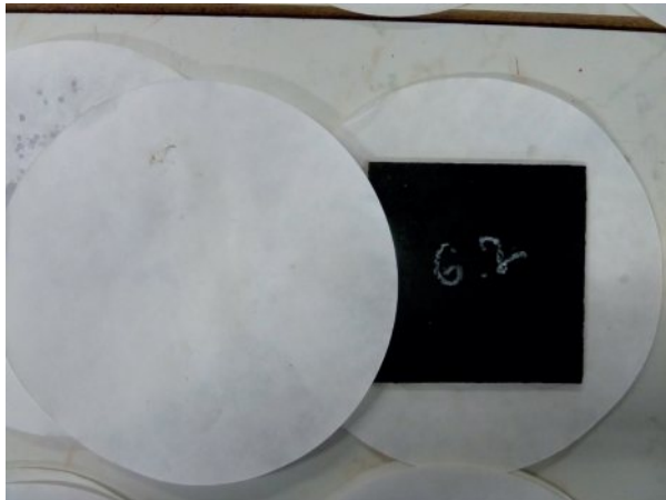
Fig. 2 Testing specimen between filter paper sheets for the water absorption test according to [2]. Source: own
