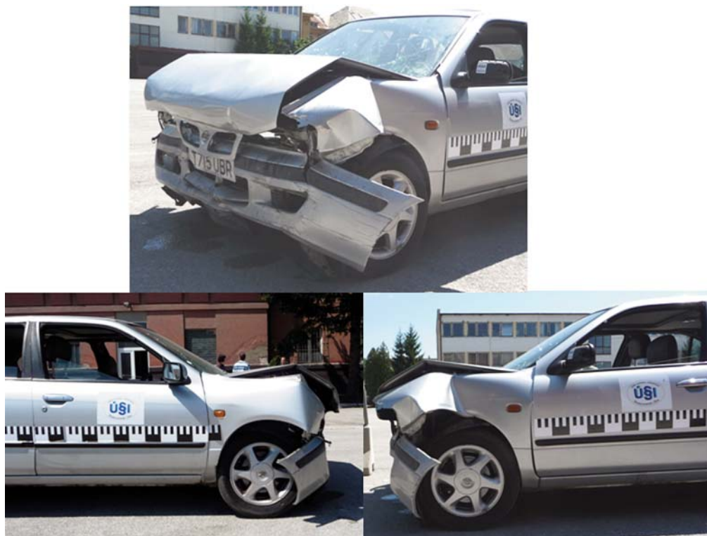
Fig. 4 Damage of the car Nissan Primera (EES = 54 km/h)
