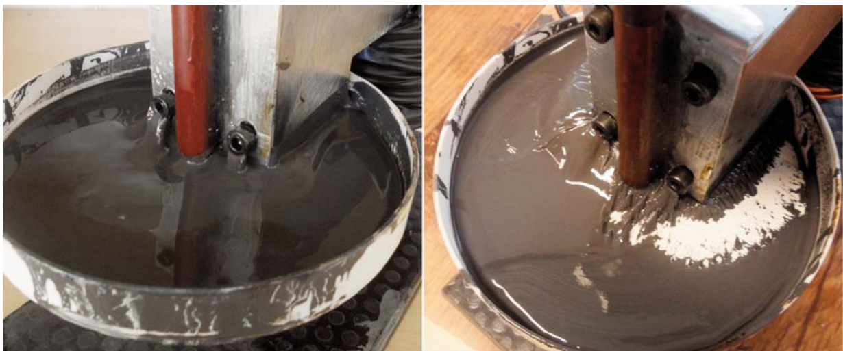
Fig. 6 Magnetorheological brake influences the viscosity of the fluid in the gap: Left - Coils are not powered; Right - Coils are powered with current density of 6 \cdot 10^4 \text{ A/m}^2
