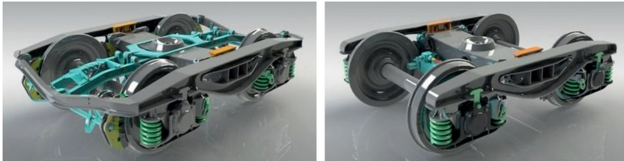
Figure 1 The original Y25 bogie (left) and the modified Y25 bogie (right)
