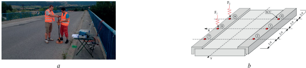
Figure 2 Modal analysis of the bridge excited by the impact load, a - impact device and its application, b - location of the measurement and loading points
