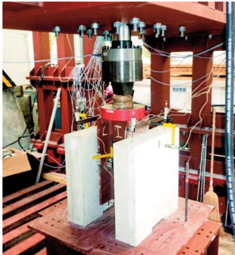
Fig. 2 Configuration of the push-out test
