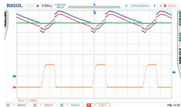
Fig. 13 Measurement signal of the LEM current sensor (red), hysteresis (blue), offset voltage (green) and gate-source voltage (orange)
