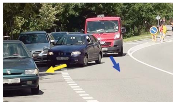
Fig. 10 Delayed vehicle after the vehicle entering the parking place by driving forward (point II; see VIDEO 03 [8])
