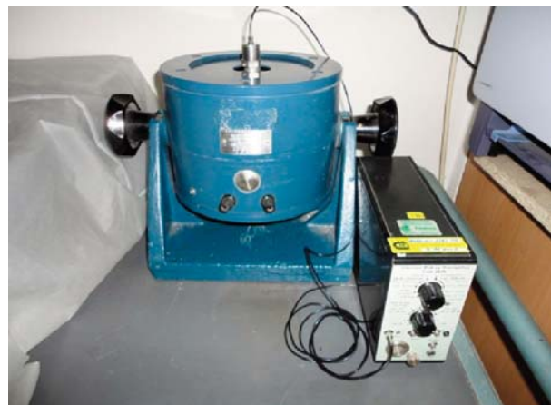
Fig. 3 Standard Vibrometer's Calibration
