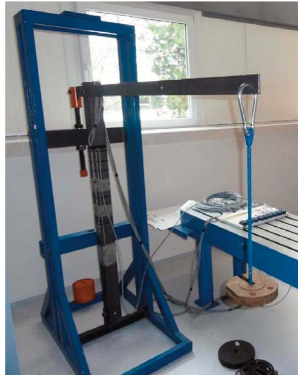
Fig. 3. The test stand to verify the installation of strain gauges and the whole measuring chain
