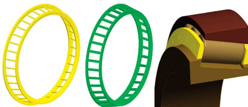
Fig. 1 Tapered roller bearing model in Pro/Engineer
