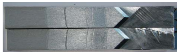
Fig. 2 "Beach" marking of crack front on specimen fracture surface
