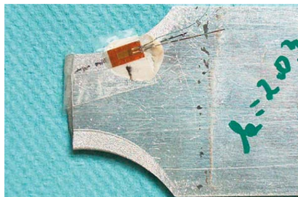
Fig. 1 Inclined position of strain gauge outside the centre of specimen with less severe shot peening
