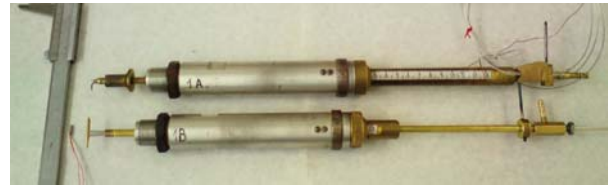
Fig. 5 Original combined probe with thermocouple (top) and new combined probe with bush for platinum thermometer (bottom)
