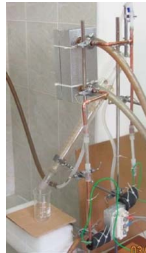
Fig. 4 Closed loop thermosyphon
