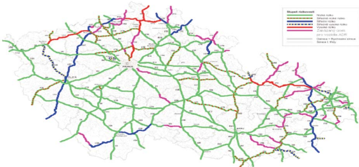
Fig. 7 Possible version of selected road network segments for dangerous goods transport with implemented exposures in the Czech Republic (pink colour – dangerous goods transport ban according to law)
