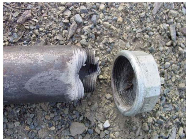
Figs. 10 and 11: Effective shooting down of the end cap from the pipe bomb
