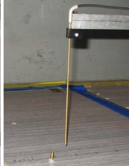
Fig. 3 Pollutant source on the floor and measuring probe
