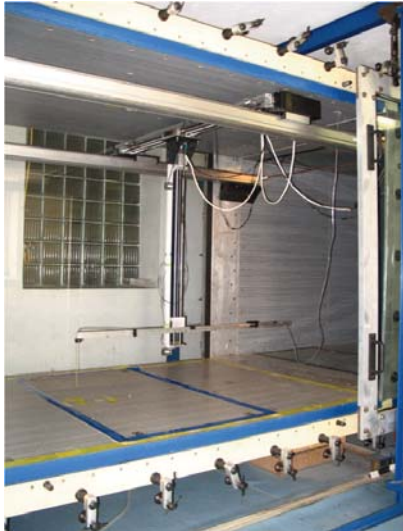
Fig. 1 Gauge section of the aerodynamic tunnel
