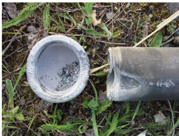
Figs. 10 and 11: Effective shooting down of the end cap from the pipe bomb
