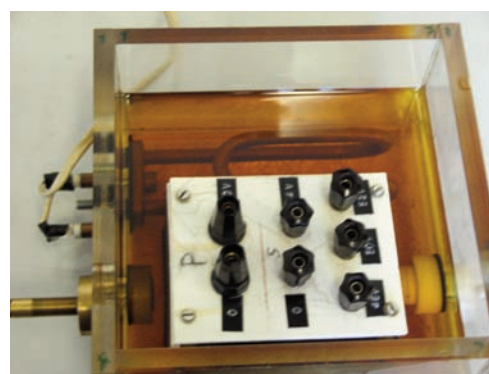
Fig. 3 Test transformer (60 VA, 220/52 V) immersed in tank with transformer oil with heating apparatus
