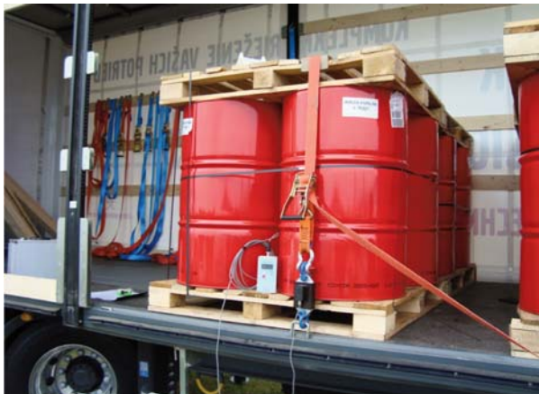
Fig. 2 Strength test of lashing bands
