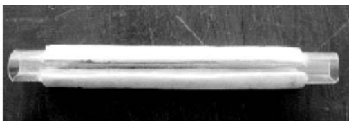
Fig. 7 Picture of glued joint specimen
