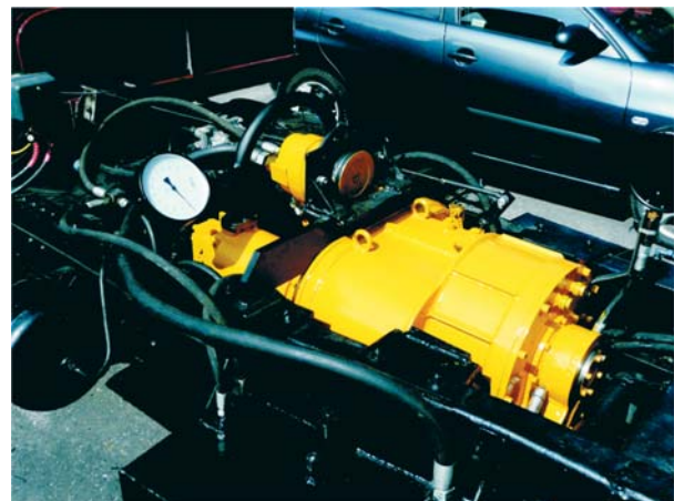
Fig. 4. The IVT 150 installed to the truck frame
