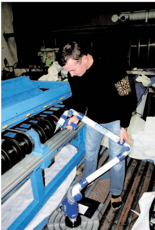
Fig. 8 Measuring of the object with FARO
