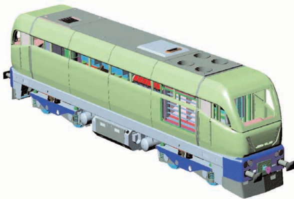
Fig. 3 Virtual parametric model based on sophisticated technologies for eContent application (diesel-electric locomotive in Pro/ENGINEER) [12]
